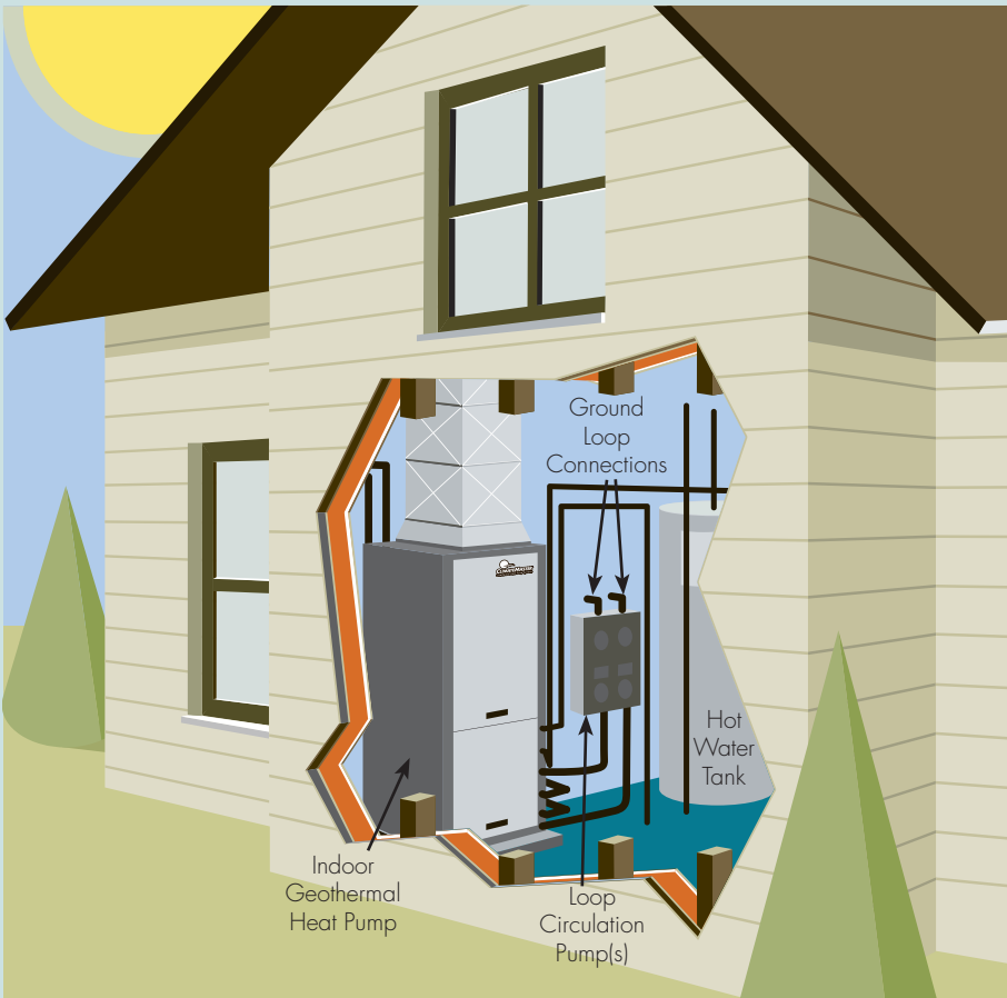
An example of a packaged upflow unit installation
